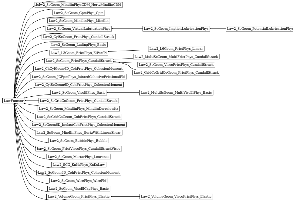
Fig. 36: Inheritance graph of LawFuncor. See also: Law2_ChCylGeom6D_CohFrictPhys_CohesionMoment , Law2_CylScGeom6D_CohFrictPhys_CohesionMoment , Law2_CylScGeom_FrictPhys_CundallStrack , Law2_GridCoGridCoGeom_FrictPhys_CundallStrack , Law2_L3Geom_FrictPhys_ElPerfPl , Law2_L6Geom_FrictPhys_Linear , Law2_MultiScGeom_MultiFrictPhys_CundallStrack , Law2_MultiScGeom_MultiViscElPhys_Basic , Law2_SCG_KnKsPhys_KnKsLaw , Law2_ScGeom6D_CohFrictPhys_CohesionMoment , Law2_ScGeom6D_InelastCohFrictPhys_CohesionMoment , Law2_ScGeom_BubblePhys_Bubble , Law2_ScGeom_CpmPhys_Cpm , Law2_ScGeom_FrictPhys_CundallStrack , Law2_ScGeom_FrictViscoPhys_CundallStrackVisco , Law2_ScGeom_ImplicitLubricationPhys , Law2_ScGeom_JCFpmPhys_JointedCohesiveFrictionalPM , Law2_ScGeom_LudingPhys_Basic , Law2_ScGeom_MindlinPhysCDM_HertzMindlinCDM , Law2_ScGeom_MindlinPhys_HertzWithLinearShear , Law2_ScGeom_MindlinPhys_Mindlin , Law2_ScGeom_MindlinPhys_MindlinDeresiewicz , Law2_ScGeom_MortarPhys_Lourenco , Law2_ScGeom_PotentialLubricationPhys , Law2_ScGeom_VirtualLubricationPhys , Law2_ScGeom_ViscElCapPhys_Basic , Law2_ScGeom_ViscElPhys_Basic , Law2_ScGeom_ViscoFrictPhys_CundallStrack , Law2_ScGeom_WirePhys_WirePM , Law2_ScGridCoGeom_CohFrictPhys_CundallStrack , Law2_ScGridCoGeom_FrictPhys_CundallStrack , Law2_VolumeGeom_FrictPhys_Elastic , Law2_VolumeGeom_ViscoFrictPhys_Elastic .
