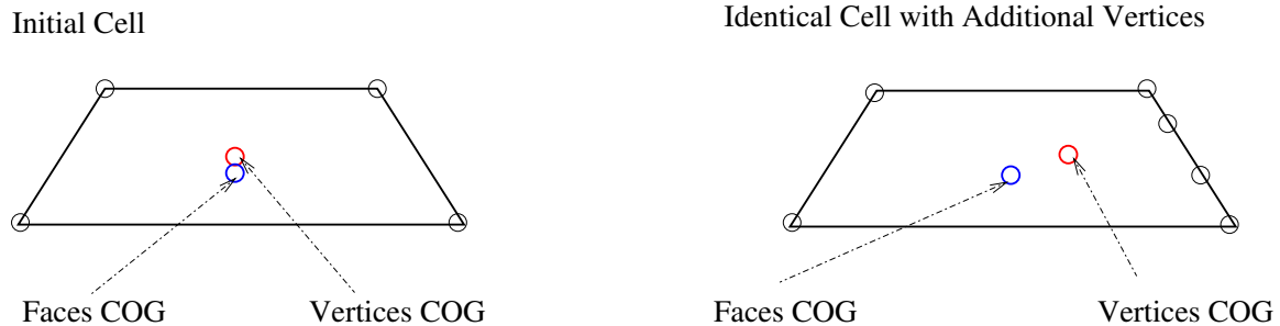
Figure VII.B.3: Choice of cell center
